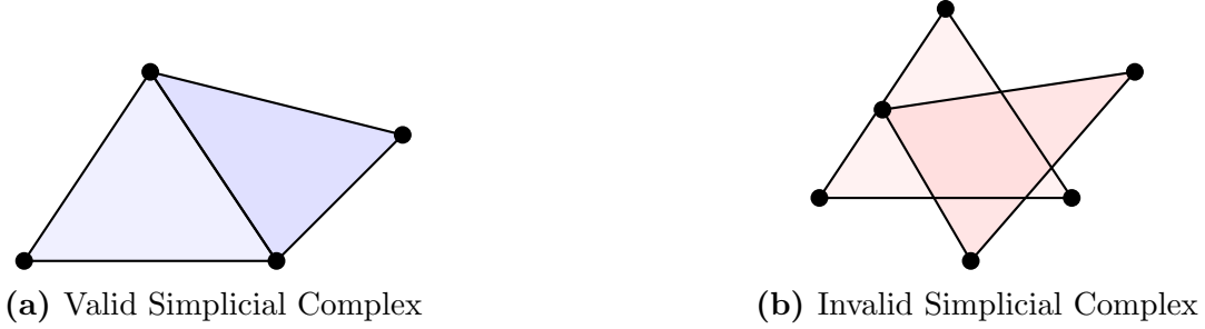
Figure 3. A comparison of simplicial intersection rules. In a valid configuration, faces meet cleanly along a shared edge or vertex. In an invalid configuration, the interiors overlap improperly without sharing face boundaries.
